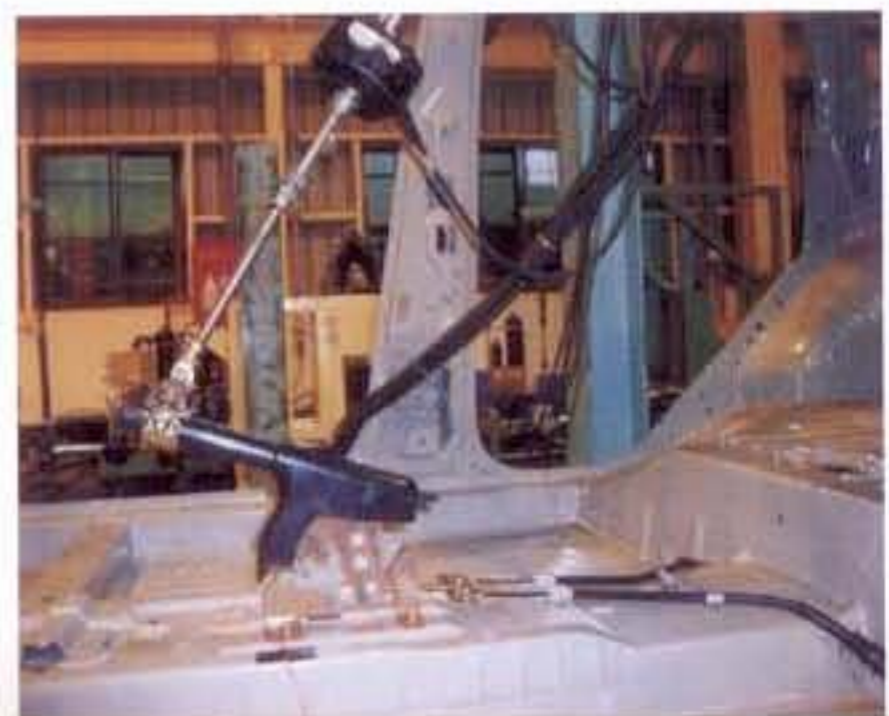
Parking Brake 操作耐久试验
